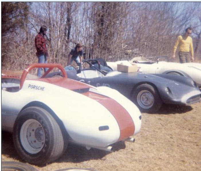
At Hobo Hill, New York about 1971. At the hill climb that day was an early 550 (right), a Devin (gray car) and a Speedster. The Mong Special was wearing reversed wheels and really wide tires, with modified wheel wells to accommodate the rubber. Below: The four-cam engine was installed in about 1961 by Floyd Sable. The rear section of the car was hinged for engine access. The front was also hinged under the nose (unlike a Porsche Spyder). Jerry Mong smiles from the cockpit of the newly-built car.
