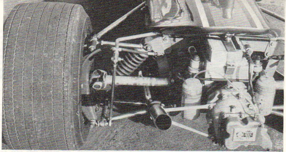
Rear suspension, with reversed lower wishbone, single top link and twin radius rod layout. The engine in the test car was peaking at 115 bhp at 9,500 rpm and had bags of torque.
